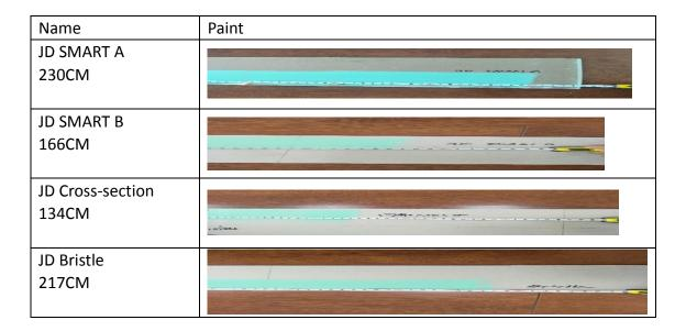
From the test, we found SMART A is painting more longer, However, it is interrupted. Not finesse and precision. JD SMART B, when release, more finesse and precision. JD Bristle, it also has interrupted
