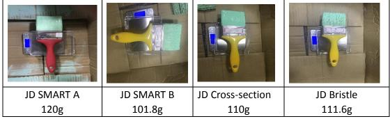
Second Step: Put them in the water-based paint for 3 minutes, Take out them until there is no paint drips and weight the paint brush
