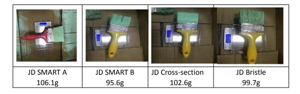
Third Step: Paint on the Gypsum board until not smooth, Weight the paint brush again
